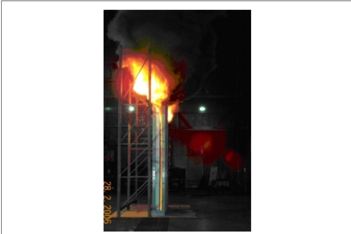
Fig. 1. Fire Test of cavity wall assembly using foam polystyrene insulation
